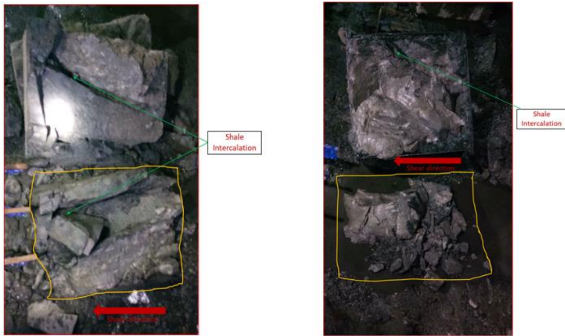
Figure 7 Toppled sandstone interface test sample
