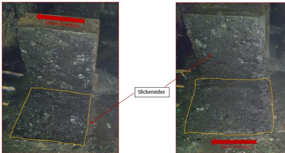
Figure 8 Toppled concrete coal interface test sample
