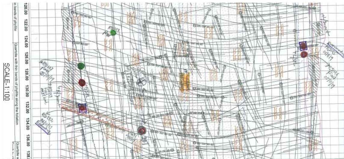
Figure 7 3D-Geological log of Power House Cavern Heading between EL 1285-1278m, showing location of Observed Confirmatory & Experimental Pull-out tests carried out on Expansion shell Rock bolts.
